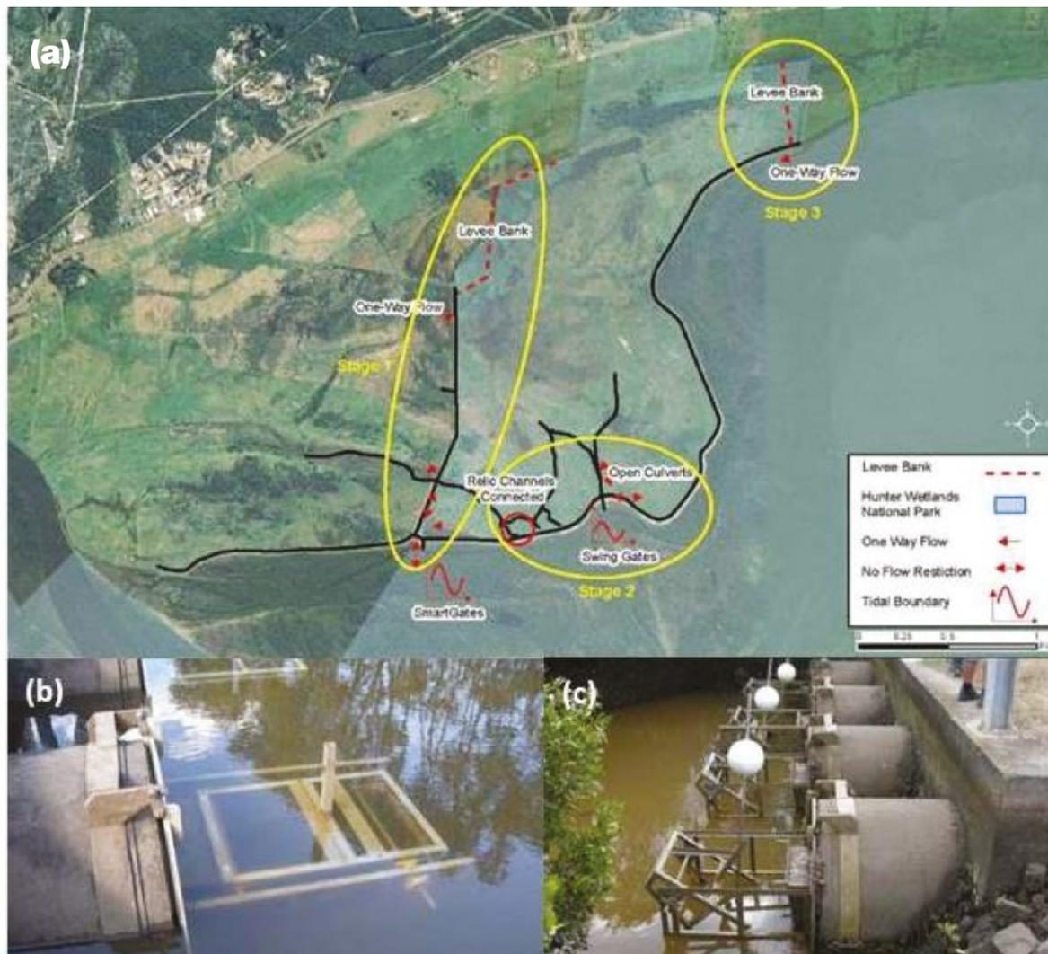
Figure 2: (a) Staged works plan for Tomago Wetland Restoration Project, and (b-c) open and closed swing gates installed as part of the Tomago Wetland Restoration Project. Source: Russell et al. 2012.
