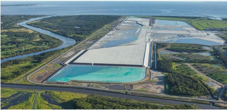
**Figure 1:** Picture of Brisbane Airport second runway under construction. New Parallel Runway site Jan 2015 – 11 million m<sup>3</sup> of sand placed to flood and climate proof the new runway. Photo: © Brisbane Airport Australia.
