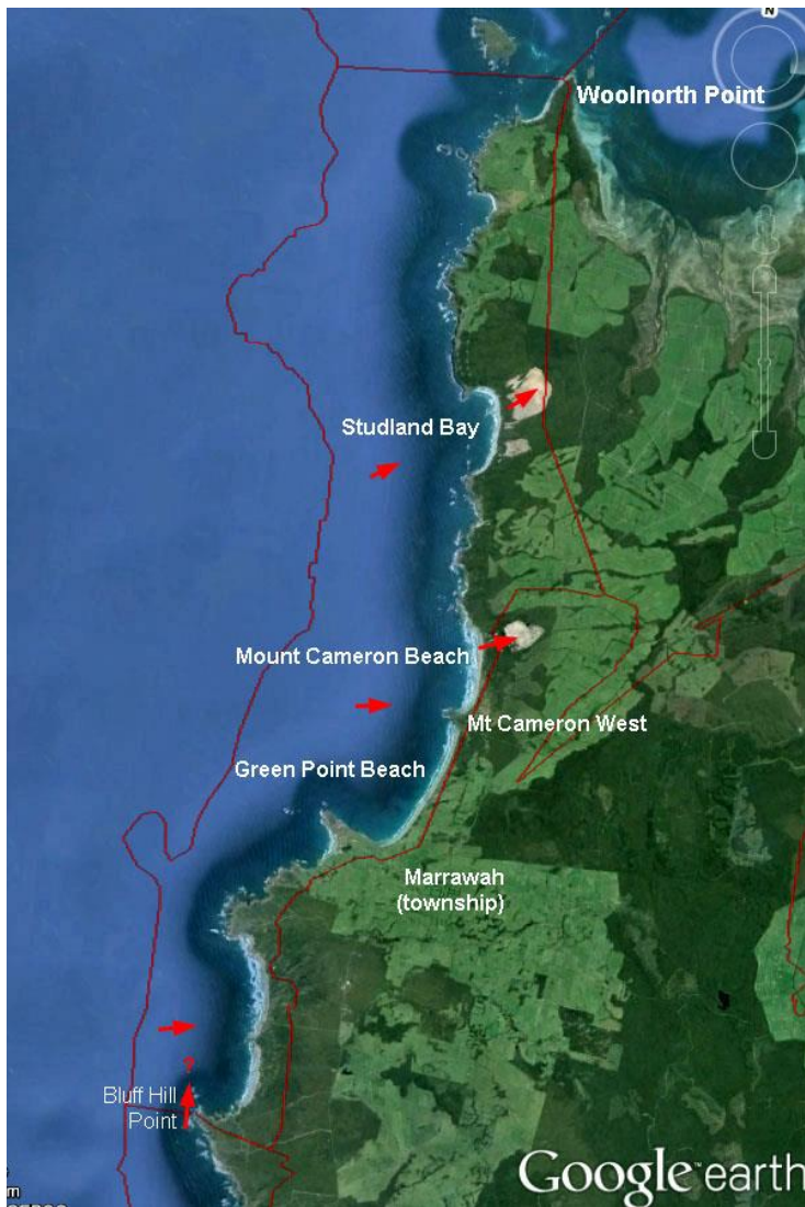
Figure 1: Compartment TAS02.03.06 Marrawah. Red arrows indicate the main inferred sediment transport pathways within this compartment. It is likely that most beach embayments in this compartment have a mostly stable or slightly gaining sand budget.
